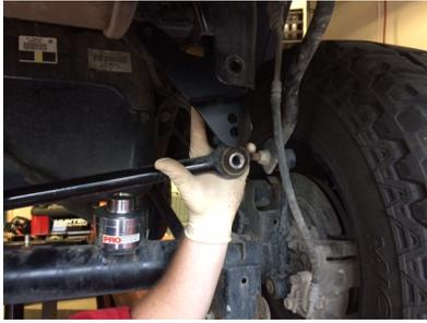
**STEP 16:** Install brake line relocater brackets on each side of vehicle using included hardware, as shown.
