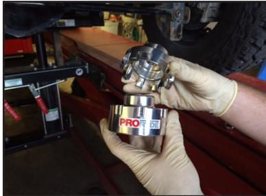
**STEP 10:** Install chosen spacers over bottom rear coil locator, and secure with included hardware, as shown.
