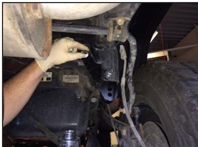
**STEP 14:** As shown, you have two available track bar anchor points. Based on the amount of chosen rear lift, determine your chosen orientation to properly center rear axle.
